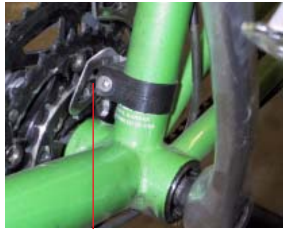
Jump stop installed
