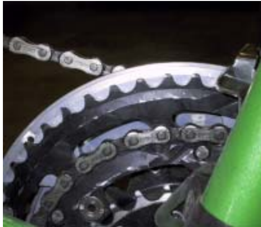
Inside view of the stoker's crank with the bash ring installed.
