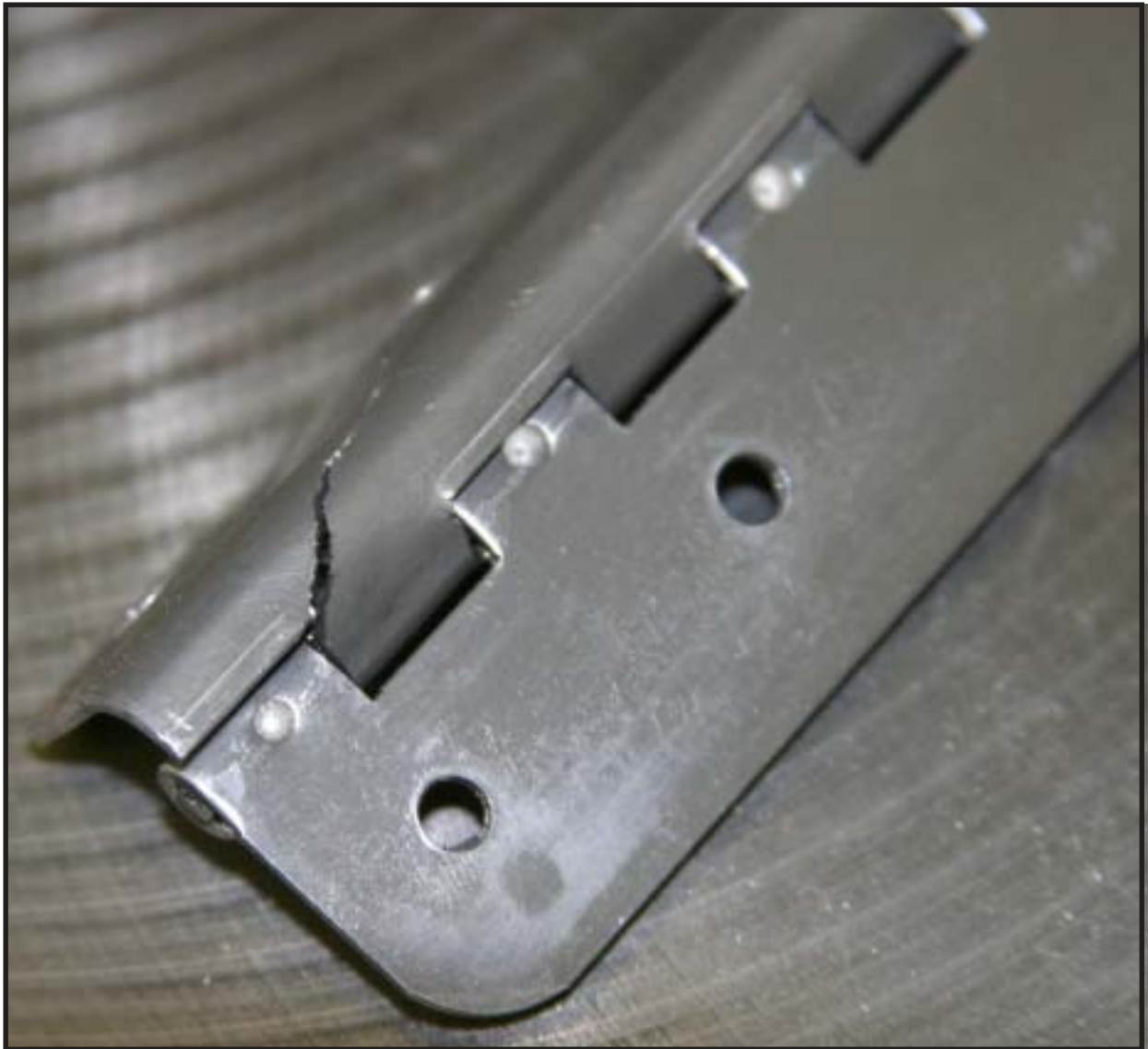
This was the hinge on the stokers seat. You can see the big crack on the left side
