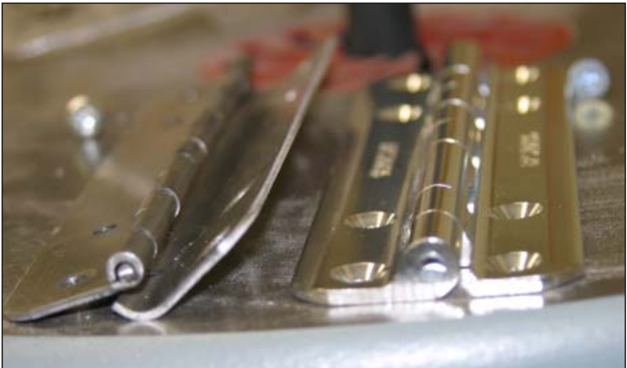
Old hinge design on the left and new on the right. Note that the old style hinge will not lay flat and is significantly thinner than the new style. The new style hinge is highly polished compared to the old style.
