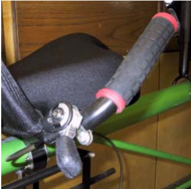
Thumb shifter mounted to the stoker's seat and used to operate the avid V brake
