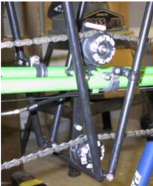
X-eyed rack secured to the chain stay with hose clamps. I used only one clamp on each side to prevent the rack from spinning.
