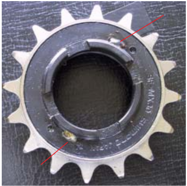
This side faces towards the bottom bracket. There are two spot welds that prevent the inside race from moving off during pedaling
