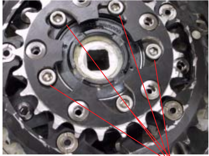
The outside plate bolts to the inside plate with 5 bolts and sandwiches the freewheel.
