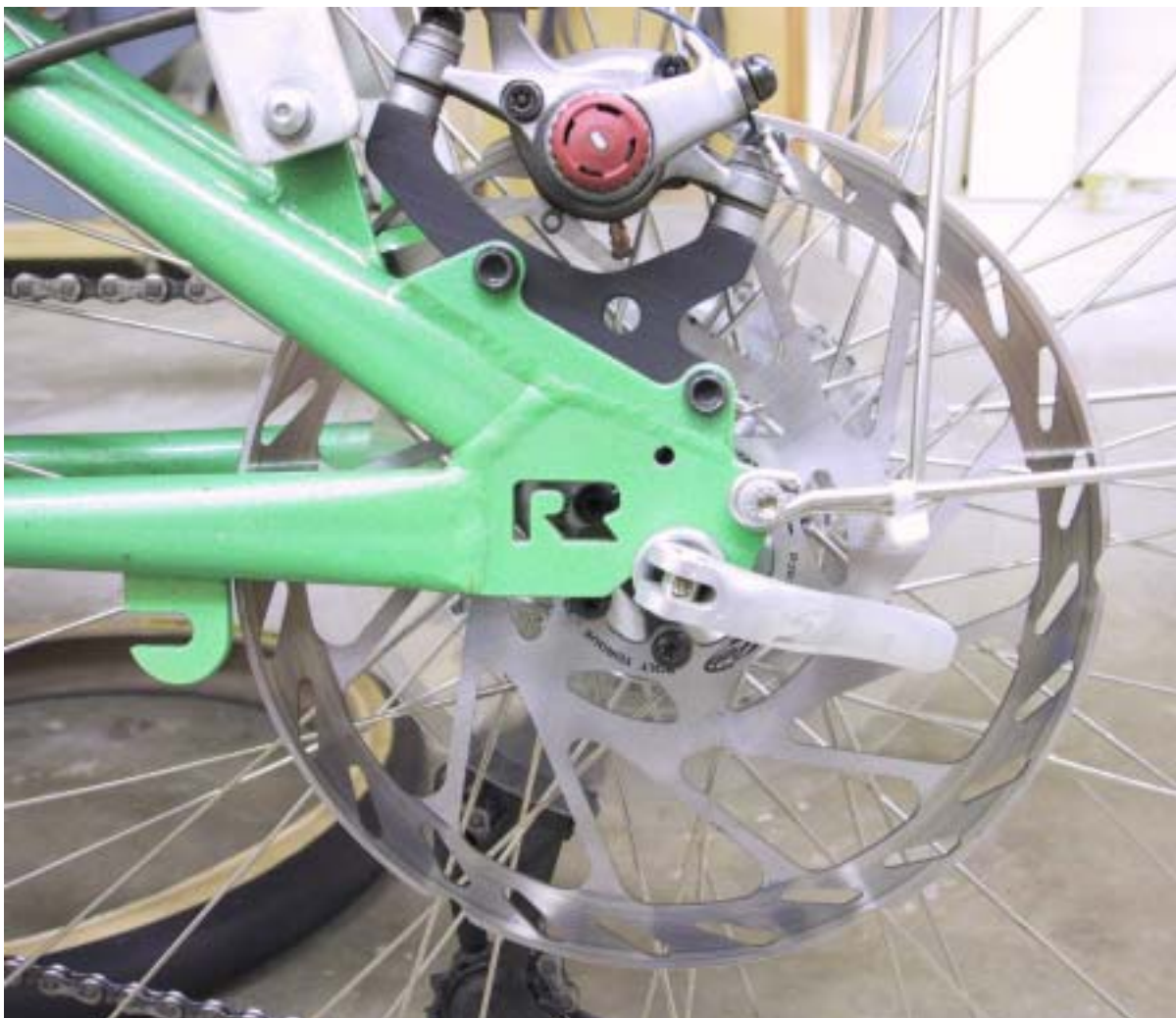
View of the rear disc brake. Note the short end on the brake cable. Avid posted a notice that the cable end should be short to prevent accidental contact with the disc.
