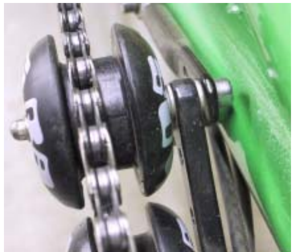
The revised L bracket installation locates the top pulley bolt close to the frame, but shouldn't be a problem
