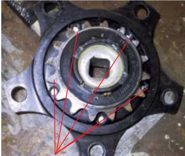
Stoker's crank sitting through the outside plate. You can see the holes where the inside plate bolts will pass through the freewheel.
