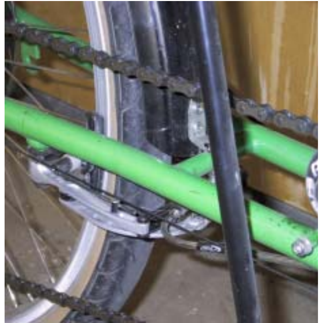
This V brake mount was already on the rear chain stay
