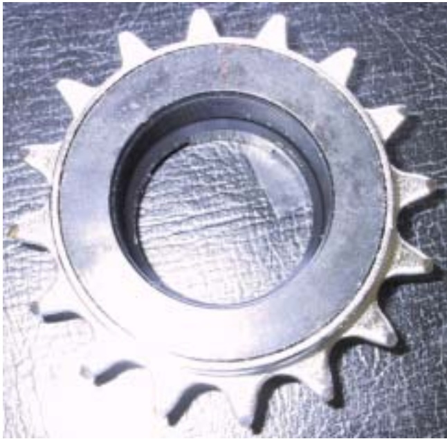
This side thread directly on to the crank and faces outside on the bike
