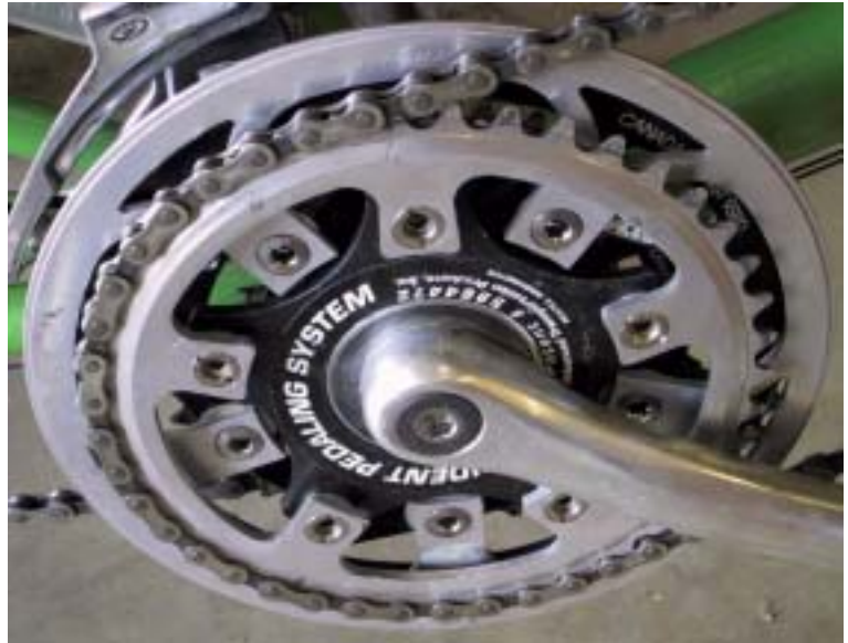
Outside view of the stoker's crank with the bash ring installed.
