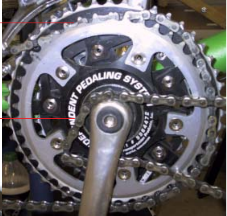
Rear chain stuck between the timing ring and big ring on the stoker’s crankset.
